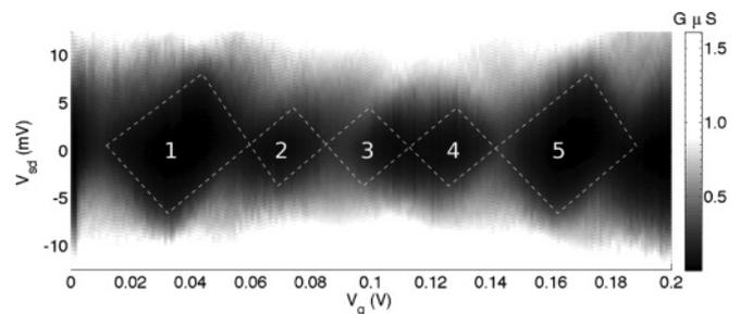
FIG. 6. Differential conductance as a function of  $V_{sd}$  and  $V_g$  of the individual (17,22) SWCNT measured at 4.3 K using standard lock in techniques with an excitation voltage of  $50 \mu\text{V}$ .
