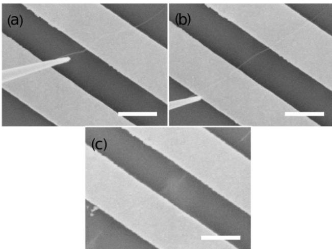
FIG. 2. SEM images showing placing of the carbon nanotube across prepatterned electrodes (Ref. 20). The scale bars represent 1  $\mu\text{m}$ .
