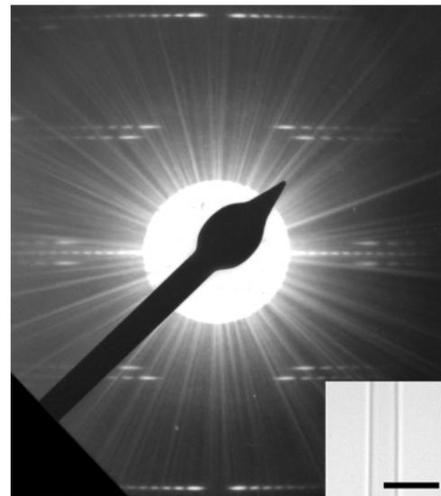
FIG. 3. Electron diffraction pattern from an individual (17,22) SWCNT and real space image (insert, scale bar represents 5 nm).
