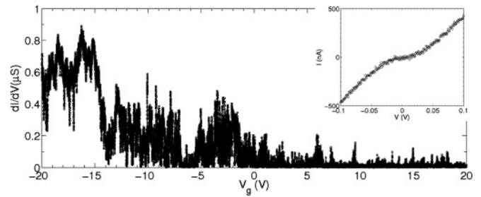
FIG. 5.  $I$ - $V$  characteristics (inset, measured at  $V_g = 0$  V) and gate voltage response of the individual (17,22) SWCNT measured at 4.3 K. The gate voltage response was measured at zero source drain voltage using standard lock in techniques with an excitation voltage of  $400 \mu\text{V}$ .
