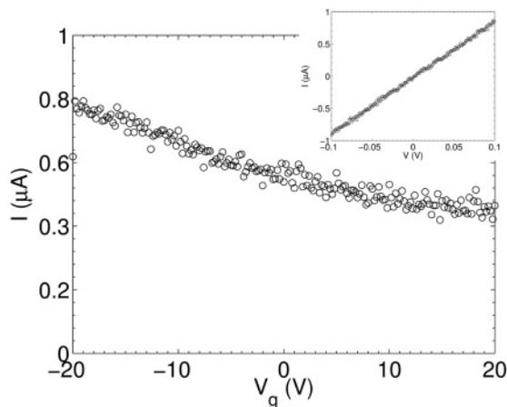
FIG. 4. Room temperature  $I$ - $V$  characteristics (inset, measured at  $V_g = 0$  V) and gate voltage response with  $V_{sd} = 100$  mV of the individual (17,22) SWCNT device.  $I$ - $V$  characteristics remain linear for all applied gate voltages between  $-20 \text{ V} < V_g < 20 \text{ V}$ .
