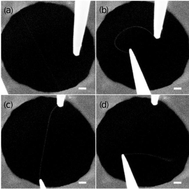
FIG. 1. SEM images showing picking of a SWCNT from the TEM grid with the tungsten STM tips (Ref. 20). The scale bars represent 200 nm.
