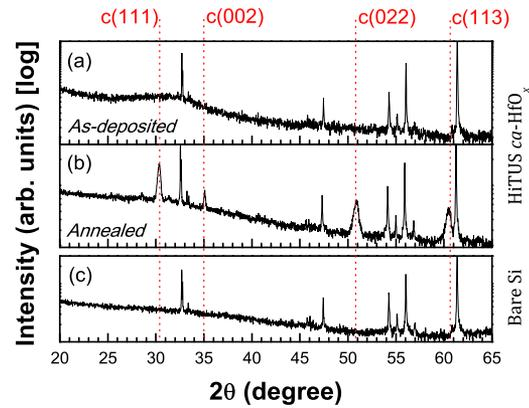
FIG. 2. (Color online) XRD scans of a typical (a) as-deposited and (b) vacuum annealed (640 °C) HiTUS  $a$ -HfO<sub>x</sub>. The broad diffraction feature around  $2\theta \sim 32^\circ$  in (a) is ascribed to amorphous HfO<sub>x</sub> while (b) matches the diffraction pattern of polycrystalline cubic HfO<sub>2</sub> (ICDD-PDF file 53-0550). (c) shows an XRD scan of a bare Si wafer for reference highlighting substrate-related reflections.
