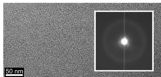
FIG. 3. A plan-view TEM image of a typical as-deposited HiTUS  $a$ -HfO<sub>x</sub> demonstrating the amorphous nature of the  $a$ -HfO<sub>x</sub> layer and the absence of nanocrystallites. An electron diffraction pattern is inset which shows diffuse halos, also consistent with the fully amorphous nature of the  $a$ -HfO<sub>x</sub> layer.
