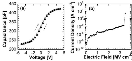
FIG. 1. (a) Capacitance-voltage characteristics and (b) leakage current density as a function of electric field for a HiTUS  $a$ -HfO<sub>x</sub> thin film (thickness  $\sim 100$  nm). Measurements were performed using an MIS (Cr-Al/ $a$ -HfO<sub>x</sub>/n-Si) capacitor structure.
