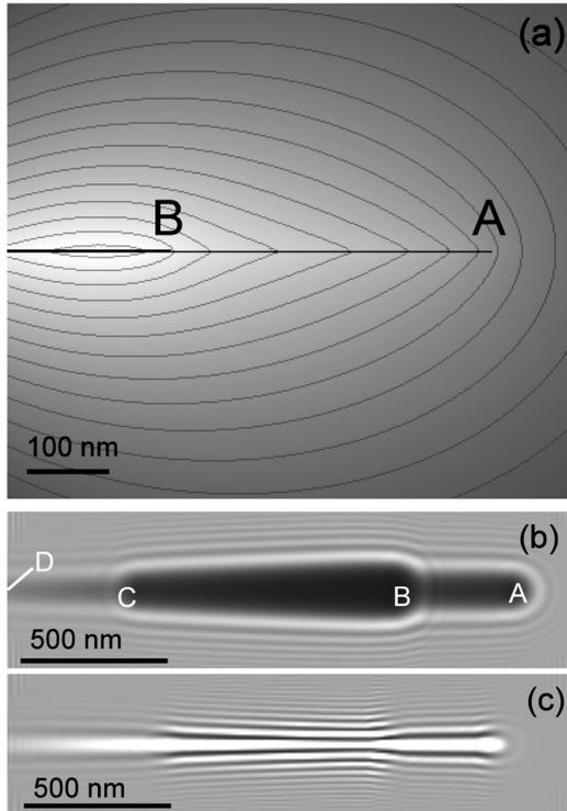
FIG. 4. (a) Simulated phase image generated by using a superposition of the terms described in Eq. (7), for the measured charge densities; the spacing of the phase contours is  $1.57 (\pi/2)$  rad. (b) and (c) corresponding simulations of defocused bright-field images of the same nanowire for defocus values of  $\pm 3$  nm, for comparison with Figs. 1(b) and 1(c). In (b) and (c) the image intensity is displayed between values of 0 and 1.5.
