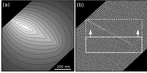
FIG. 2. (a) Phase shift measured using off-axis electron holography from the square region marked in Fig. 1(b) for an applied electrical bias between the nanowire and the counterelectrode of 50 V. The contour spacing is 1.57 rad. (b) Laplacian of (a). The annotations in (b) indicate the rectangular regions used to determine the cumulative charge along the wire.
