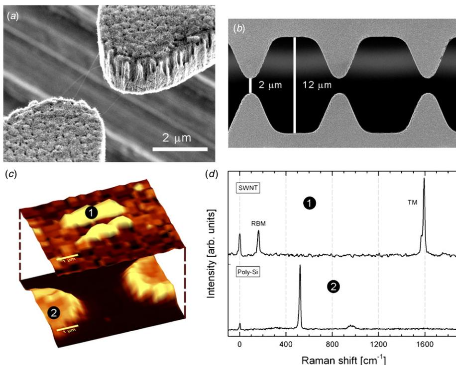
**Figure 4.** (a) SEM image of three SWNTs spanned between a pair of closely spaced poly-Si tips. (b) Demagnified SEM from (a) to show the tip definition. (c) Raman image of the same tip pair as shown in (a). (d) Representative snapshots showing SWNT and poly-Si-specific phonon modes in the Raman shift.
