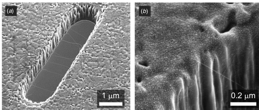
**Figure 2.** (a) SEM of a rectangular hole from the surface micromachined grid with aligned SWNT bridges. (b) Zoomed SEM image showing catalytic Ni particles and a SWNT bridge.
