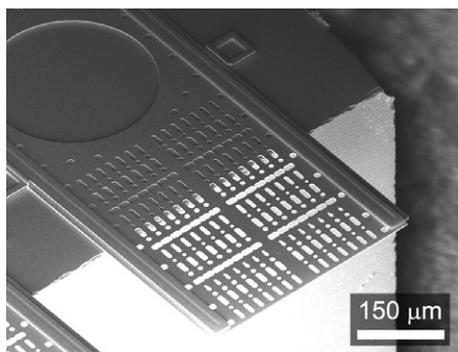
**Figure 1.** SEM image of a silicon microchip containing a surface micromachined grid slit off the chip edge.
