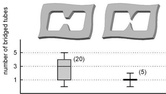
**Figure 6.** Box plot of two different tip apex geometries. Figures in parenthesis indicate the number of measured tip pairs. The ultra-sharp tips have a mean number of spanned SWNT of 1 tube per tip pair.
