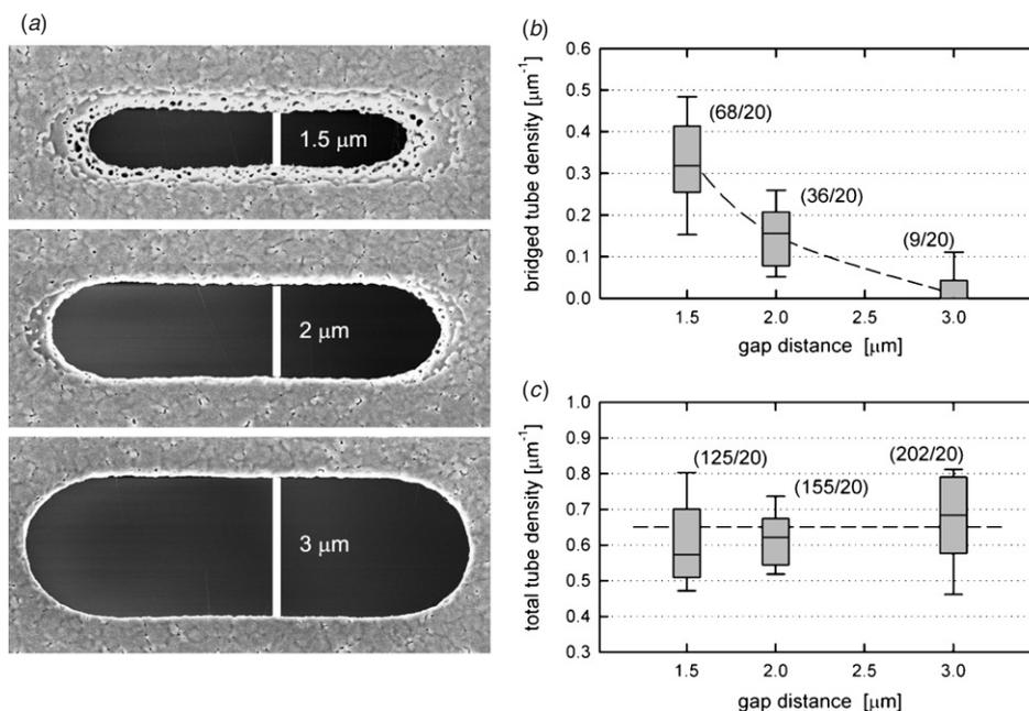
**Figure 3.** (a) SEM of rectangular holes of different gap sizes, (b) tube bridge density across different gap sizes. Figures in parenthesis indicate the number of measured tubes which successfully bridged over the gaps (tube bridges/gaps). (c) Total tube density in the same gaps. Figures in parenthesis indicate the number of measured tubes grown inside the gaps but which did not necessarily lead to a bridge (tubes/gaps).
