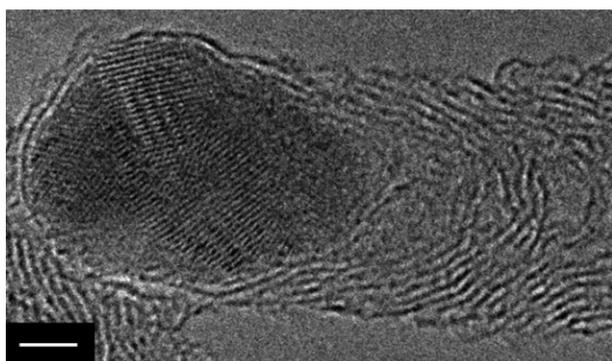
**Fig. 3** HRTEM image of an individual CNF from the sample shown in Fig. 2. Scale bar is 2 nm.
