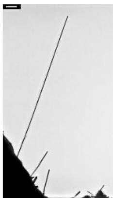
Fig. 2. TEM image of as-grown nanocrystals on edge of 300 mesh Mo TEM grid (scale bar 1  $\mu\text{m}$ ).
