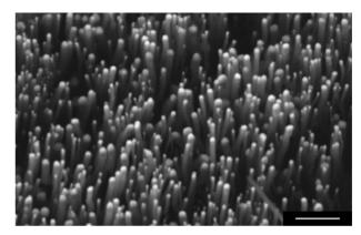
Fig. 1 SEM image of CNFs grown Co colloid, flocculated and centrifugated once. Cobalt catalyst particles are visible in the tips of the CNTs. 400  $^{\circ}$ C, NH<sub>3</sub>: C<sub>2</sub>H<sub>2</sub> 200: 50 sccm. Scale bar 500 nm.
