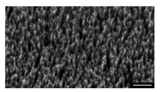
Fig. 2 SEM image of carbon nanofibres grown from Co colloid, flocculated and centrifugated twice. 300  $^{\circ}$ C, NH<sub>3</sub>: H<sub>2</sub>: C<sub>2</sub>H<sub>2</sub> 200: 200: 100 sccm. Scale bar 250 nm.
