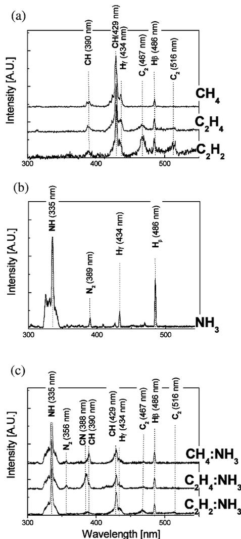
Fig. 1. Optical emission spectra of a 600 V dc discharge for (a) pure hydrocarbons, (b) pure ammonia and (c) hydrocarbons in ammonia dilution used for nanofibre growth.
