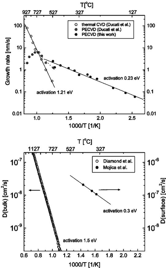
Fig. 6. (a) The CNF growth rate variation with temperature for thermal CVD and PECVD with  $\text{C}_2\text{H}_2/\text{NH}_3$ . The data points for thermal CVD and high temperature PECVD are from previous data by Ducati et al. [14]. (b) Temperature dependence of carbon diffusion in nickel from data by Diamond et al. [17] and Mojica et al. [18]. The values for the activation energies were calculated from a linear interpolation of the slopes.
