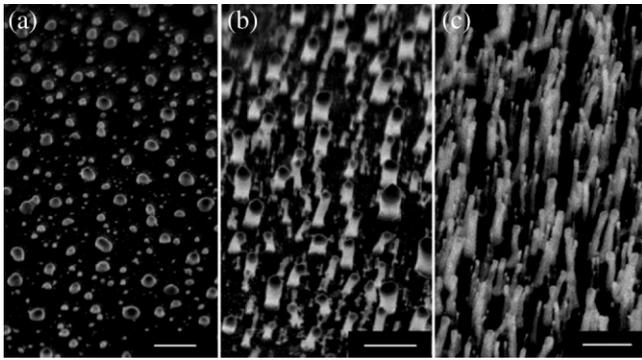
Fig. 2. SEM photographs of a nickel catalyst film after exposure to an ammonia-diluted (a) methane, (b) ethylene and (c) acetylene plasma (flow ratio 1:4) at 450 °C and 1.5 mbar for 10 min (scale bars: (a), (b), (c) 500 nm).
