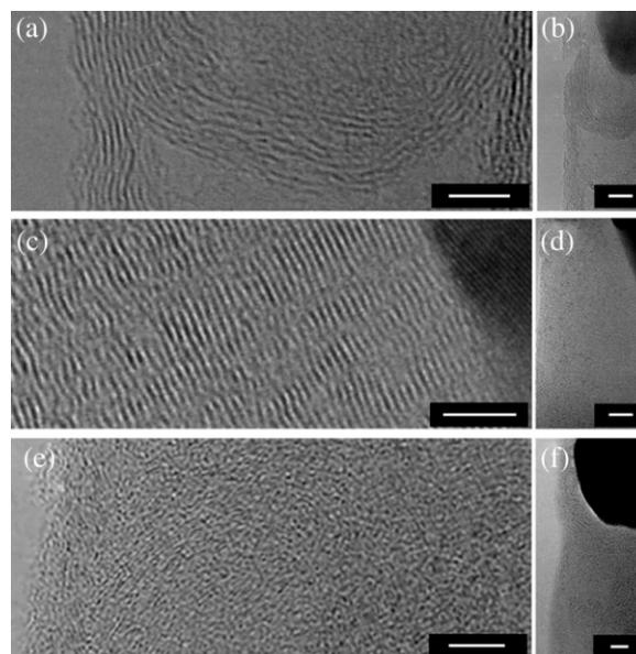
Fig. 5. TEM images of CNFs deposited with diluted acetylene at 500 °C [(a),(b)], 390 °C [(c),(d)] and 270 °C [(e),(f)]. Images (a),(c) and (e) are close-ups of (b),(d) and (f), respectively, (scale bars: 5, 10, 5, 15, 10 and 15 nm, respectively).
