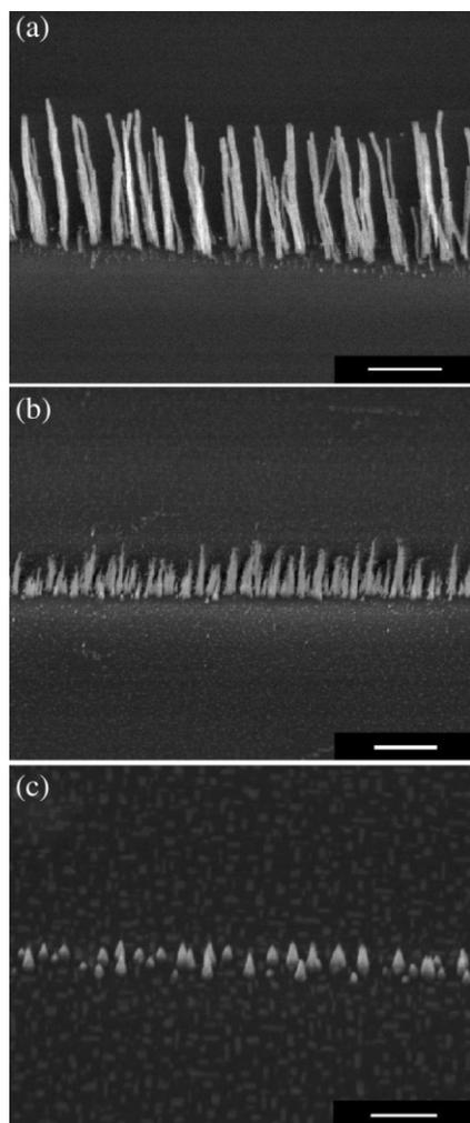
Fig. 4. SEM photographs of vertically aligned CNFs grown with diluted acetylene from e-beam patterned Ni lines at (a) 500 °C, (b) 270 °C and (c) 120 °C. A tilt angle of 40° was used for imaging (scale bars: (a), (b) 1  $\mu\text{m}$  and (c) 500 nm).
