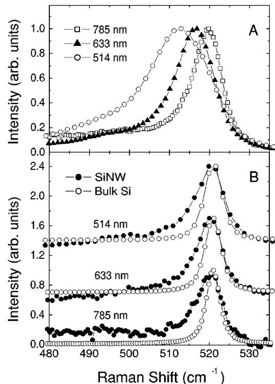
FIG. 3. (a) Evolution of SiNW Raman spectra with excitation wavelength for similar laser powers of  $\sim 3$  mW. (b) Comparison of SiNW and bulk Si spectra measured at the same low power ( $\sim 0.02$  mW) for 514-, 633-, and 785-nm excitation wavelengths.
