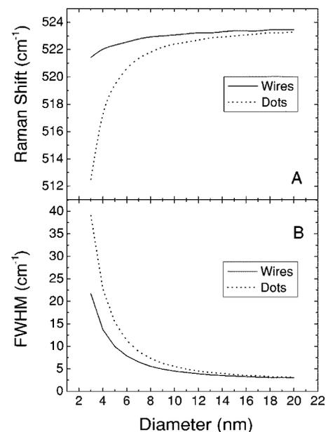
FIG. 1. Calculated trends for (a) peak position, (b) FWHM for Si wires and dots of decreasing dimensions.
