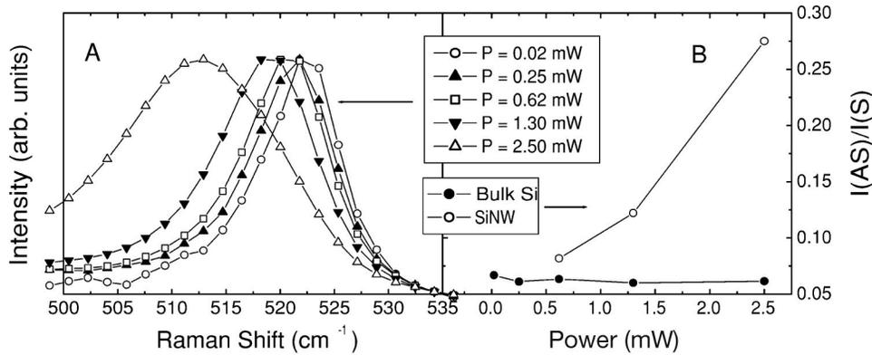
FIG. 2. (a) SiNW Raman spectra at 514.5 nm for increasing laser power. (b)  $I(AS)/I(S)$  as a function of laser power for SiNW and bulk Si.
